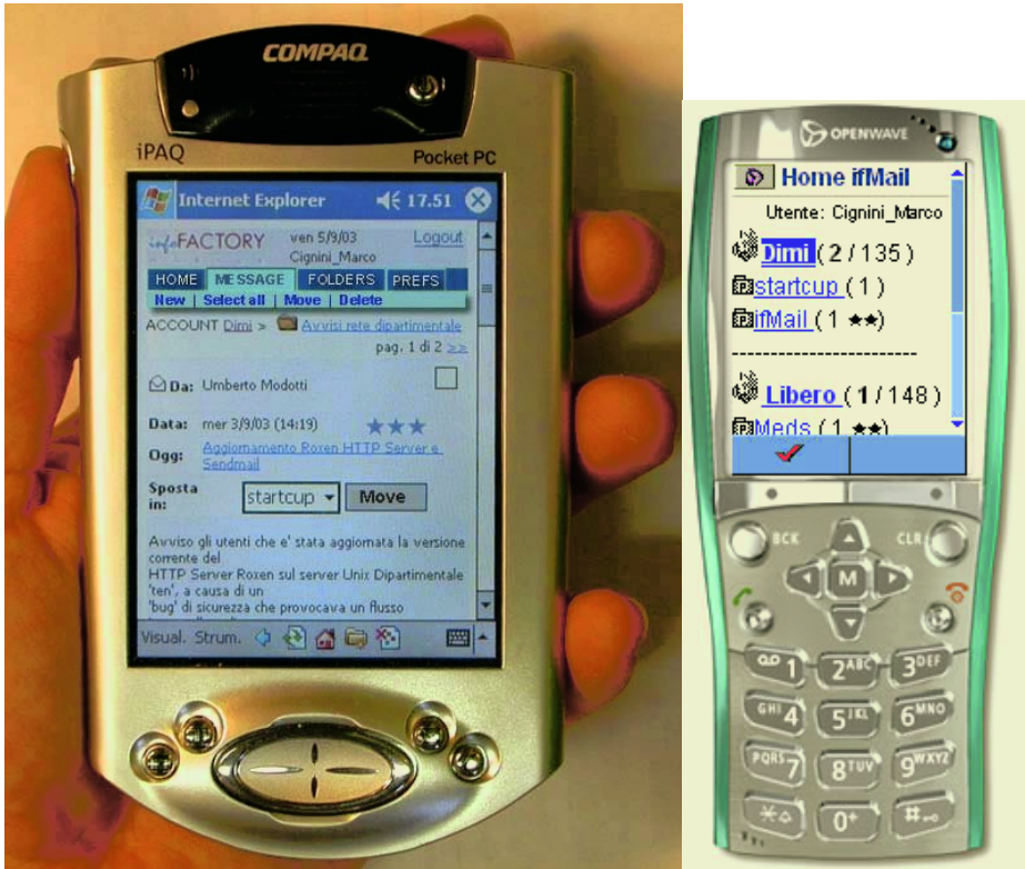
Fig. 4. ifMail user interface: email reading on a PDA (left) and folders of new categorized messages on an Openwave WAP phone simulator (right).
