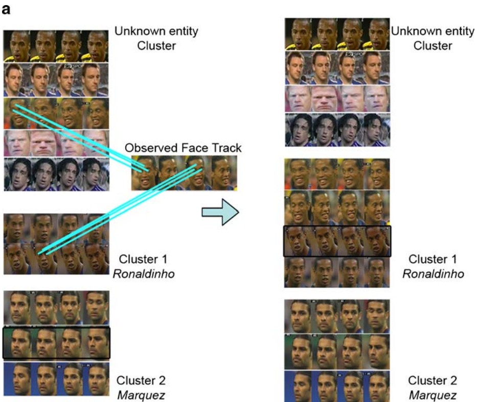
Fig. 3 Two examples of instance clustering and cluster updating, respectively applied to a face image sequences, obtained from face detection and tracking, and b highlight shots, obtained from video segmentation. As a new face/highlight sequence is presented, it is associated with the nearest instance in the clusters (SIFT matching and highlight descriptor matching are used respectively for faces and highlights, as explained in Section 4) and clusters are updated accordingly. Cluster splitting is shown for highlight clusters as an effect of cluster updating
