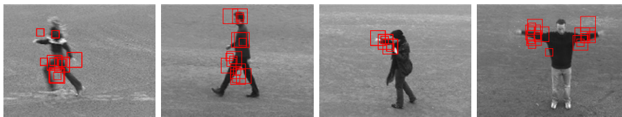
Fig. 4. Examples of space-time interest points extracted at multiple scales for different actions. Clips are taken from the KTH dataset: running, walking, boxing and hand-waving.
