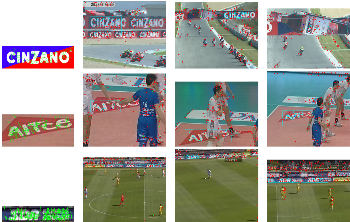
Figure 1.8: Some example matches. The leftmost column contains the trademark model annotated with its detected SIFT feature points. The other three columns contain a portion of a video frame where a match was found. Points indicated in cyan are those selected as “good” matches according to equations (1.3, 1.4).
