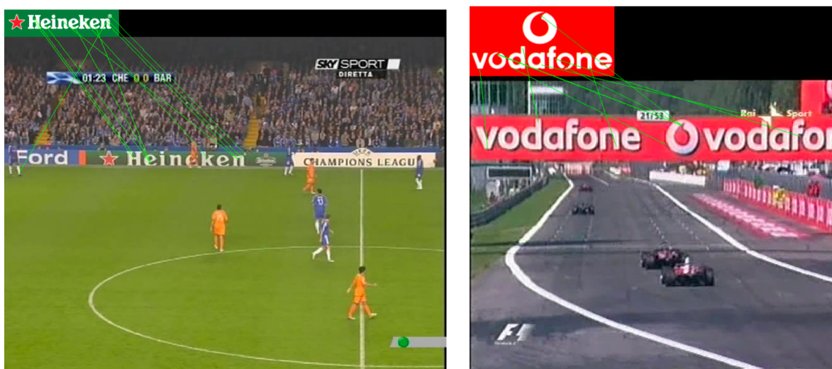
Figure 1.6: Two examples of the “traditional” SIFT matching technique.
